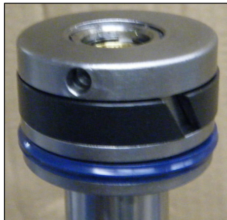
Figure 11: Piston with Wear Ring Installed
