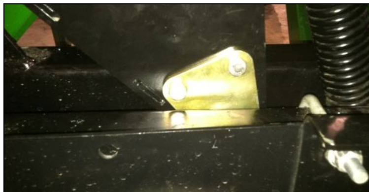
Figure 5: Upper Pin Installed
