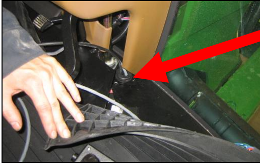
Figure 18: Hole under Floor Mat
