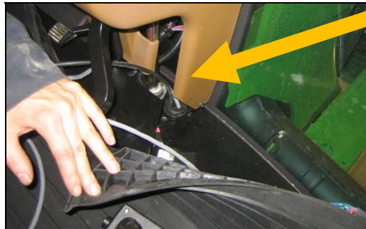
Figure 19 – Hole under Floor Mat
