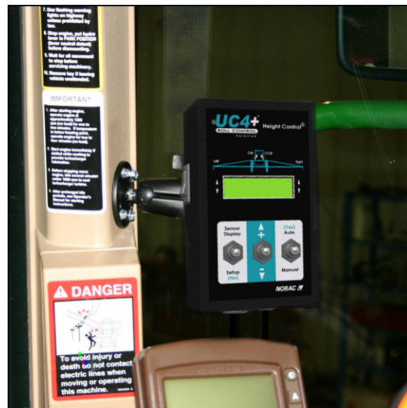
Figure 30: JD Control Panel Mounting
