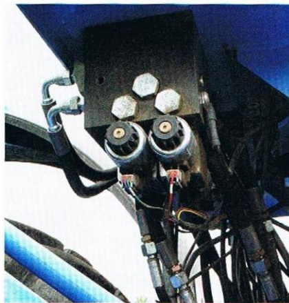
In the case of the solution of a retrofitting „Total Control“ one additional proportional valve block will be mounted.
