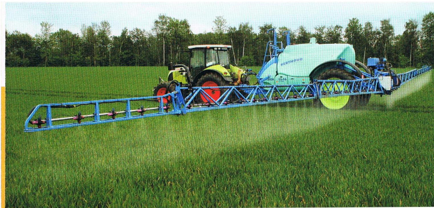
The ultrasonic height control for spray booms from Norac was here retrofitted
