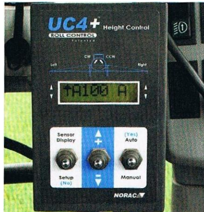
With the use of the small control panel the automatic spray height control „Total Control“ from Norac will be activated and set.
